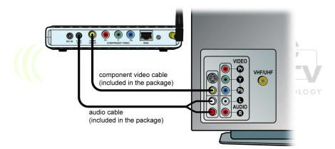
Ocnnect the power adapter to the InternetVue<sup>™</sup> DC power jack input first (a), then plug in the power adapter into an AC outlet (b). Turn on your TV or projector and select the appropriate AV input. If your configuration involves a wired connection to the InternetVue<sup>™</sup>, go ahead and connect it to your router using an Ethernet cable.
